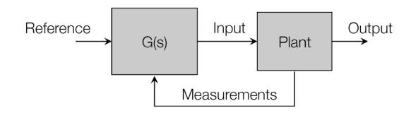
The classical controller is replaced by an optimization algorithm:
