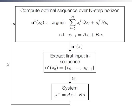
For unconstrained systems, this is a **constant linear controller**However, can extend this concept to much more complex systems (MPC)
