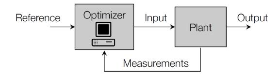
The optimization uses predictions based on a model of the plant.
