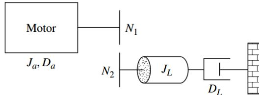
$$\frac{\theta_m(s)}{E_a(s)} = \frac{K_t/(R_a J_m)}{s + \frac{1}{J_m}(D_m + \frac{K_t K_b}{R_a})} \rightarrow \left( J_m, D_m, \frac{K_t}{R_a}, K_b \right)$$
