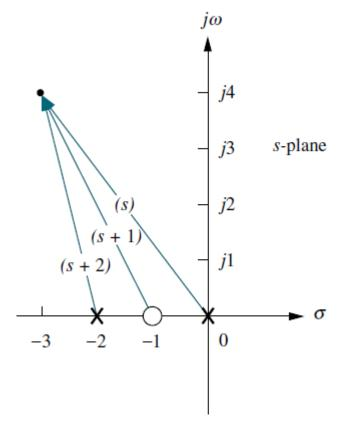
$$M \angle \theta = \frac{\sqrt{20}}{5\sqrt{17}} \angle 116.6^{\circ} - 126.9^{\circ} - 104.0^{\circ} = 0.217 \angle - 114.3^{\circ}$$
