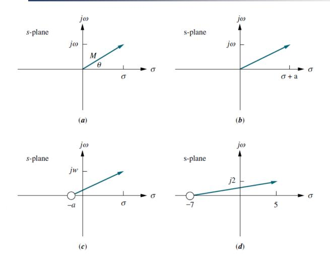
**FIGURE 8.2** Vector representation of complex numbers:  $\mathbf{a} \cdot s = \sigma + j\omega$ ;  $\mathbf{b} \cdot (s+a)$ ;  $\mathbf{c} \cdot \text{alternate}$  representation of (s+a);  $\mathbf{d} \cdot (s+7)|_{s \to 5+i2}$
